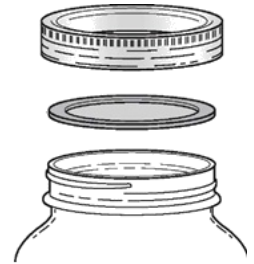
Use threaded, tempered glass jars that accept 2-piece closures.
